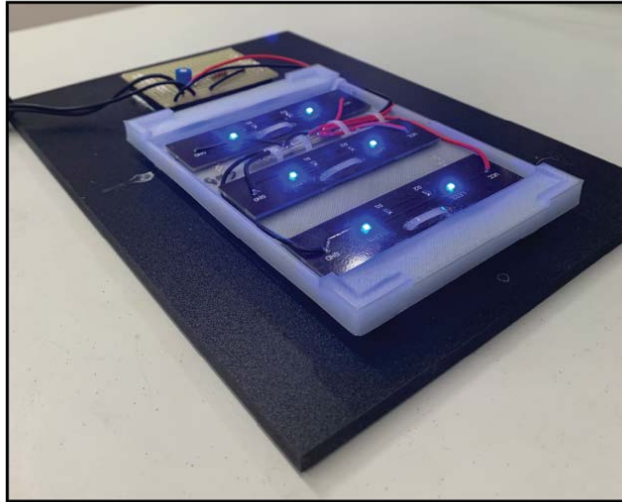
Figure 32. A blue light illumination plate used to activate Cry2 in fixed cell assays.
